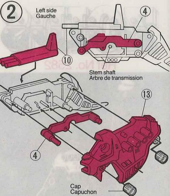
Set part (10) in place first, then attach part (13). Set part (4) so that it comes on top of the stem shaft.
